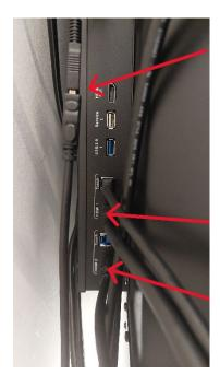
USB connection cable: for the permanently installed camera, extension, runs through the wall cable guide to the fixed computer. The laptop comes with a USB extension cable that can be connected to the upper cable for temporary use of the camera with a laptop. Afterwards, please re-establish the cable connection as shown here.
